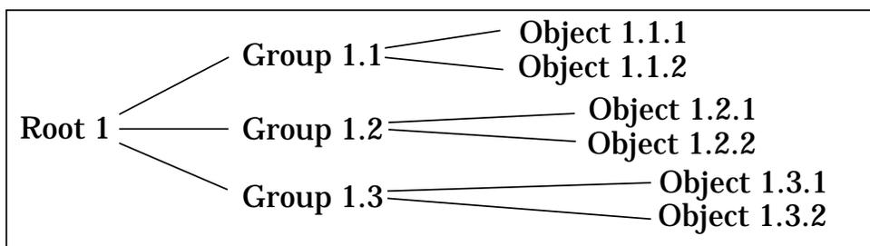
Figure 6-1. Hierarchical MIB Tree Structure
