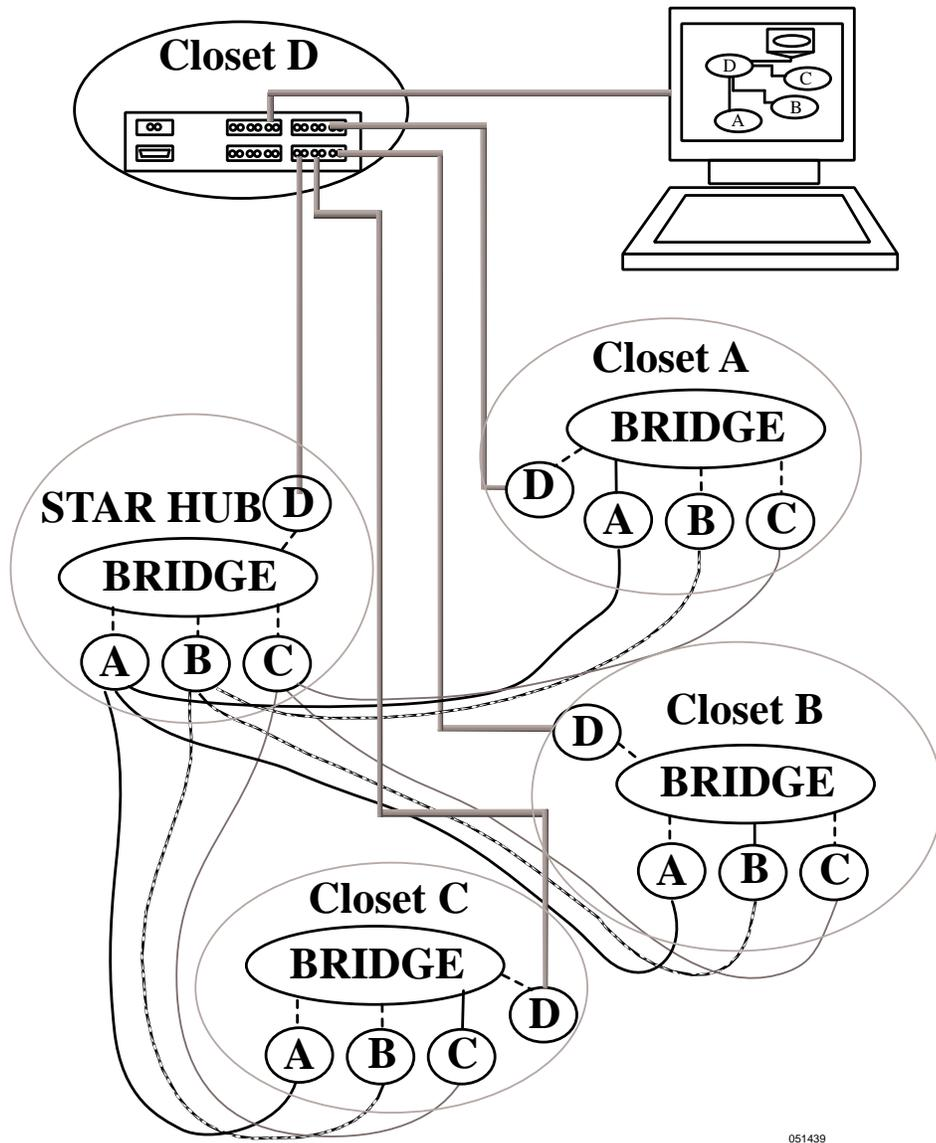
Figure 2-7. Configuring a Fault Tolerant Wiring Scheme
