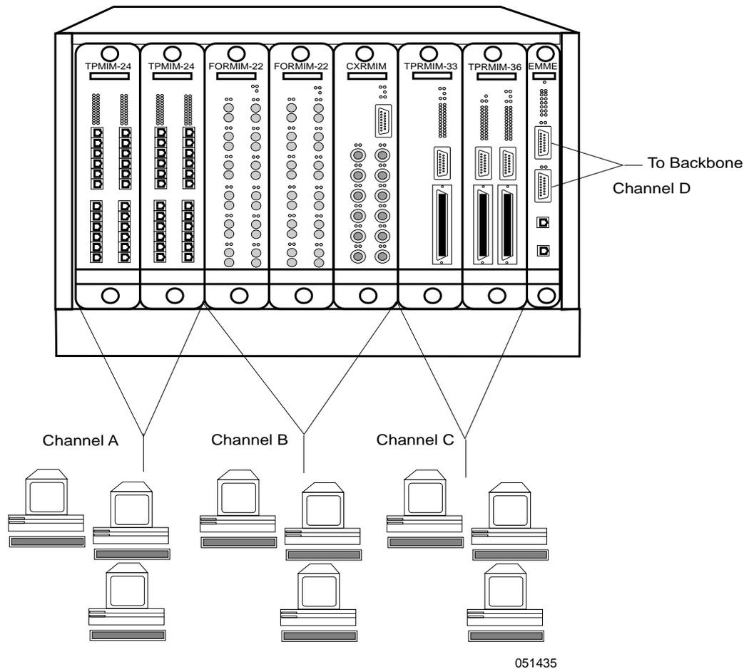
Figure 2-3. Single MMAC-FNB Configuration
