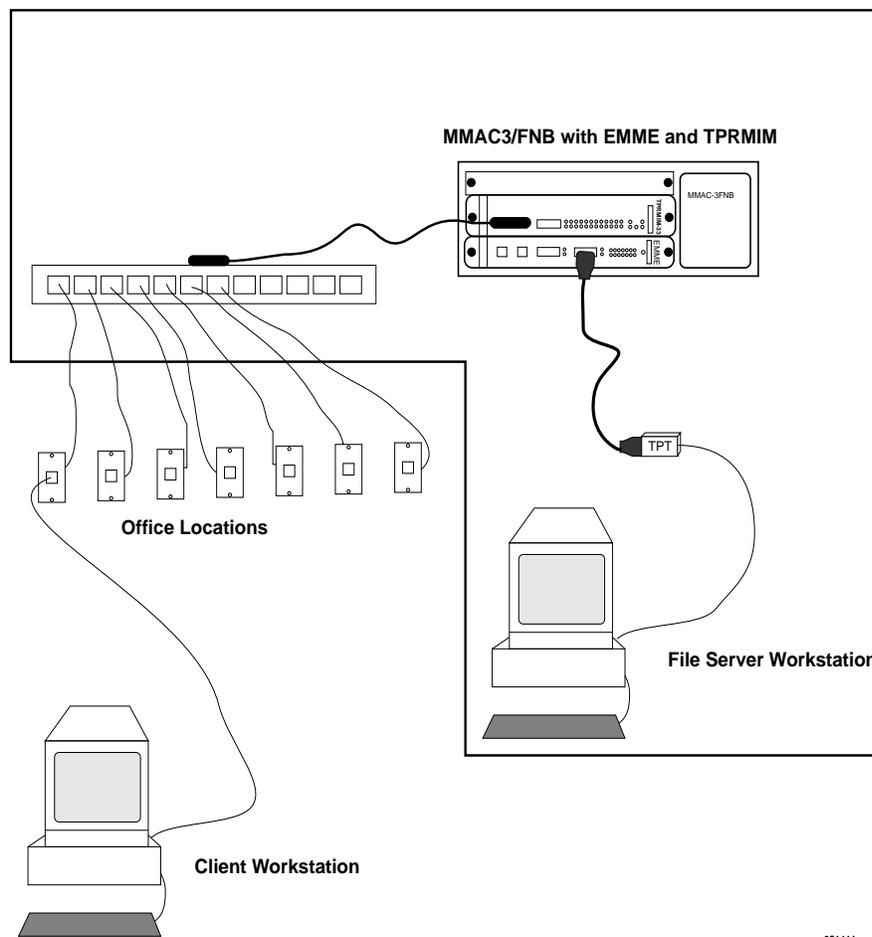
Figure 4-2. Installation Check-Out Test Configuration
