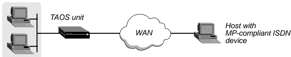
Figure 55. Multilink PPP (MP) connection
