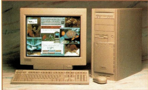
Tatung's COMPstation U10/300 is an Ultra 10-compatible with Ultra Wide SCSI on the motherboard instead of EIDE, giving it a potential 40-MB/s throughput to disk.
