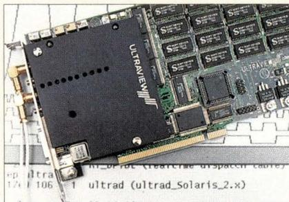
and concurrent with, the A/D samples. Each board also has four TTL outputs, which can provide a high-speed stream of digital data vectors at the same rate as the D/A samples. Incoming A/D samples are automatically stored in the board's dual-ported 4 MB of RAM and D/A samples are automatically outputted from the same RAM software. The software, which is supplied with the ULTRAD-1280, allows waveforms to be displayed in Xview or to be continuously stored or retrieved from disk.
