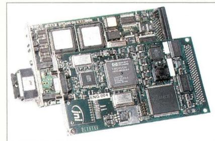
FibreStar supports all Fibre Channel connection modes, including Class 1, Class 2, Class 3 and Intermix. It can handle data over point-to-point, arbitrated loop and switched network topologies. FibreStar supports Solaris 2.4, 2.5 and 2.6. FibreStar Model FC64-1063-CI costs \$3,150 and FibreStar Model FC64-1063-NOI costs \$3,675.
