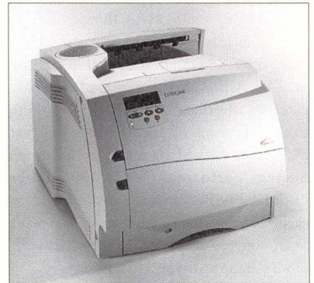
To avoid printing bottlenecks, the Optra S printers include VR-4300, 64-bit MIPS RISC processor-to-high-speed PCI-bus MarkNet network adapters, advanced data management and optimized controller architecture. The Optra S printers continue to offer 1200-by-1200-dpi and a 1200 Image Quality mode.
