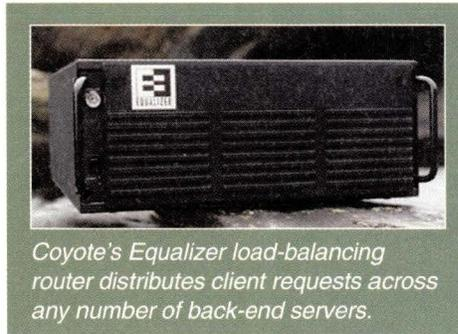
*Coyote's Equalizer load-balancing router distributes client requests across any number of back-end servers.*
