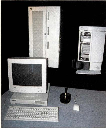
the company says. MPS 2 comprises the MPS multiprocessor controller; premastering software, which formats the data-to-CD-R requirements; two 4x CD-Recorders; a media autoloader; and an inline printer. MPS 2 is compatible with major UNIX platforms, including Solaris, AIX, HP-UX, Digital UNIX, IRIX and SCO UNIX. Pricing starts at \$47,100, depending on configuration.
