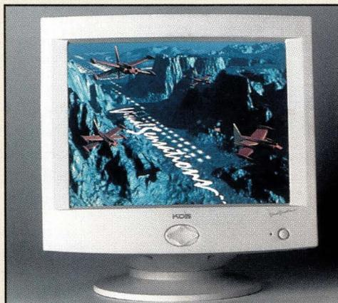
1,600-by-1,200 pixels at a 79-Hz refresh rate. KDS uses a super-fine crystal pigment cathode ray tube (CRT) from Matsushita Electric Industrial Co. to produce a .26 mm dot pitch.
