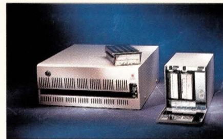
refined to provide 25 GB of native capacity per drive with a native data transfer rate of 3 MB/s.
