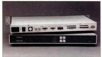
The unit's fiber-optic interface incorporates Apcon's SC optical connectors, which convert SCSI data into a 1.06-Gb/s Fibre Channel serial data stream, transmitted on the fiber-optic interface to a remote PowerLink for conversion to the appropriate SCSI signals.
