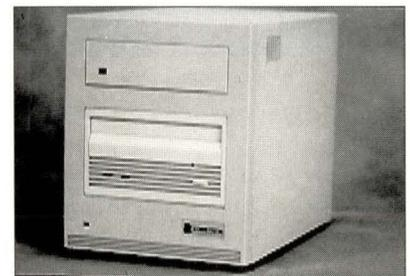
MB of RAM as well as task manager and firmware modules. SPANStor is a stand-alone, plug-and-play storage controller that includes a SPANControl printed circuit board, enclosure and appropriate SCSI devices.
