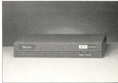
Computer. The Danube sits in a remote office LAN and provides a WAN interface. On the LAN side, the Danube comes with autosensing Ethernet connectors to link to 10BaseT via an RJ-45 connector, or to 10Base-5 via an AUI connector. On the WAN side, the product supports such WAN interfaces as RS-232, V.35, RS-422, X.21, as well as ISDN Basic Rate Interface.
