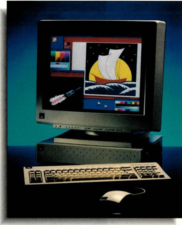
*The DataStation 30, from Pinnacle Data Systems, is a SPARCstation 20-compatible based on one or more hyperSPARC processors. Pinnacle is a relative newcomer to the SPARClike market although it has a long history in the refurbished Sun market.*
