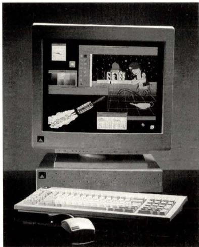
DataStation 20 comes in single-, dual- and quad-processor models. It is based on the 50-MHz and 60-MHz versions of the SuperSPARC.
