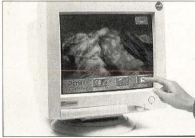
The company says the IntelliTouch may find roles in applications such as public information kiosks, process control and computer-based training. The monitor has a 1,280-by-1,024 resolution and a vertical refresh rate of up to 100 Hz. Pricing begins at \$1,980.
