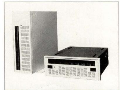
RAID controller. The SA-H335 comes in tower and rack-mount configuration. In either design, the product supports eight hot-plug drive slots with steel canisters for the disk drives. It also has dual redundant hot-pluggable power supplies, a fast/wide SCSI interface, automatic drive bay power sequencing, support for multiple SCSI hosts, mounting and power for a RAID controller and an optional 3½-inch tape/optical drive canister.
