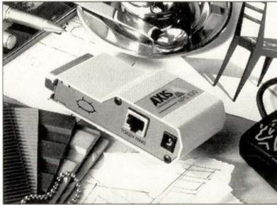
ETRAX chip, a 32-bit device that provides both a token-ring and an Ethernet controller. The NPS 630 and 632 control the token ring by providing simultaneous printing of Novell Inc.'s NetWare, LAN Manager, LAN Server, TCP/IP and Microsoft Corp.'s NT.
