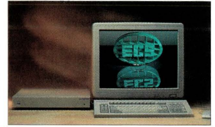
The VS-2000 from Elitegroup Computer Systems Inc. is one of several new 40-MHz SPARClikes.
