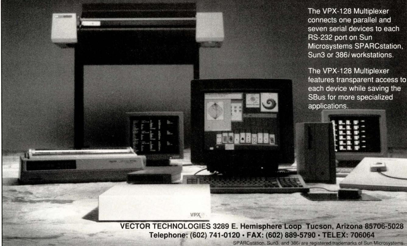
The VPX-128 Multiplexer connects one parallel and seven serial devices to each RS-232 port on Sun Microsystems SPARCstation, Sun3 or 386i workstations.
