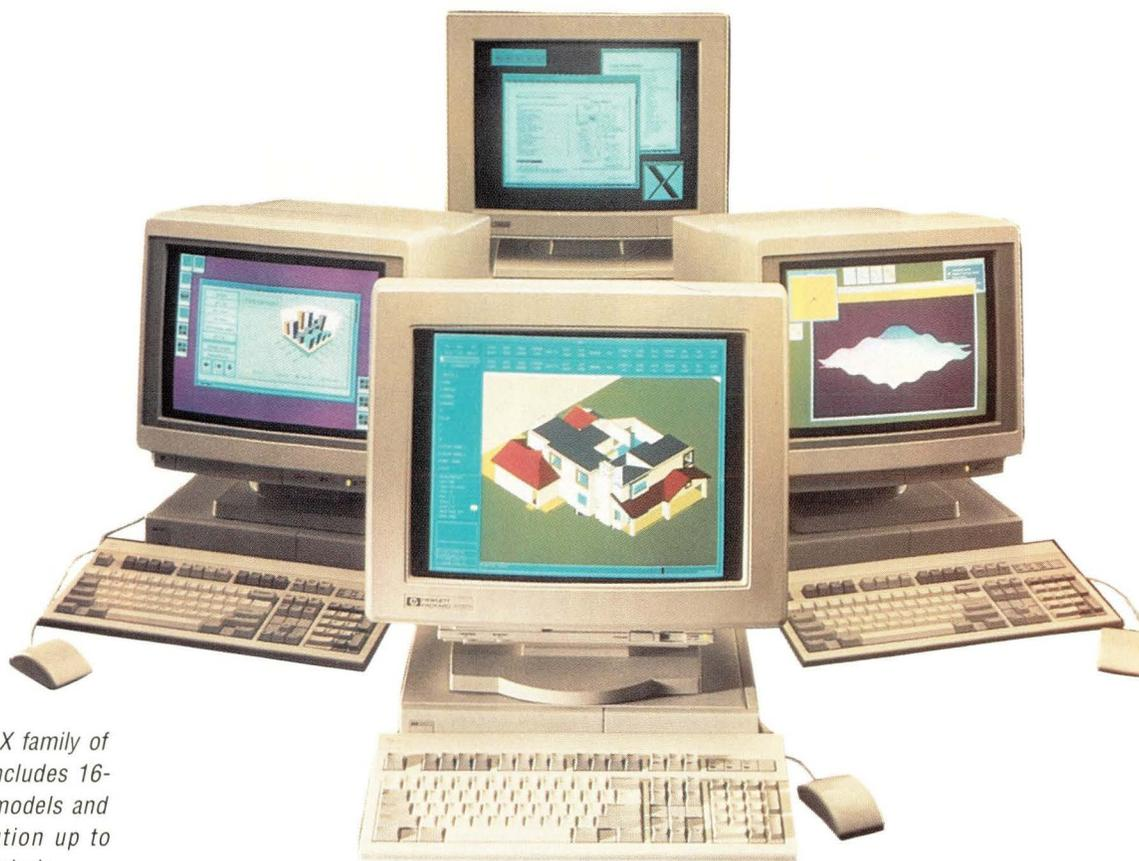
The HP 700/RX family of X-terminals includes 16- and 19-inch models and offers resolution up to 1280 by 1024 pixels.
