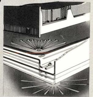
In the MADDbox Zero Footprint™ Series a unique universal power supply supports the entire range of inputs from 100 to 260 Volts, and **each device — disk or tape — has its own individual power supply.** Failure of a power supply will, therefore, not disable an entire subsystem.
