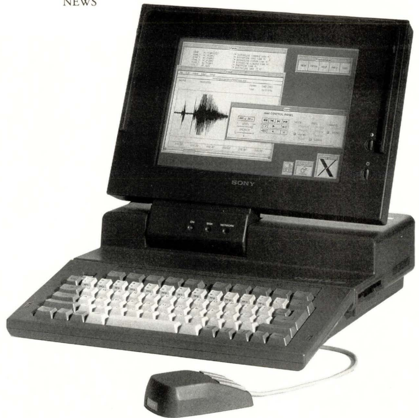
Sony Microsystems Co.'s NEWS 3250 laptop workstation is the first MIPS-based portable. But RDI may not be far behind with its own MIPS-like.
