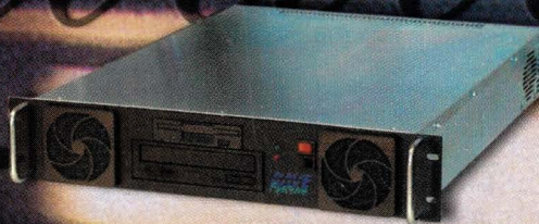
Rave Systems RackMount-2UAXi Original Sun® UltraAXi in 2U chassis.
