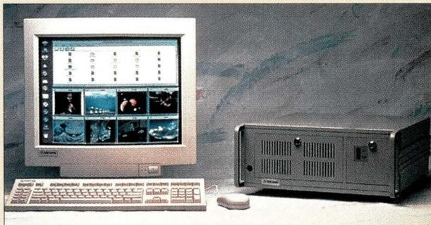
a 64-bit Ultra Port Architecture (UPA) slot is available for add-ons such as Creator3D or Elite3D graphics cards. Other standard features include two serial ports, one parallel port and a 100BaseT Ethernet interface.
