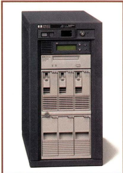
The SureStore HD Server 4000 is HP's first foray into the network-attached storage market. The new system connects directly to Ethernet LANs and offers 18 to 90 GB of RAID 5 storage.
