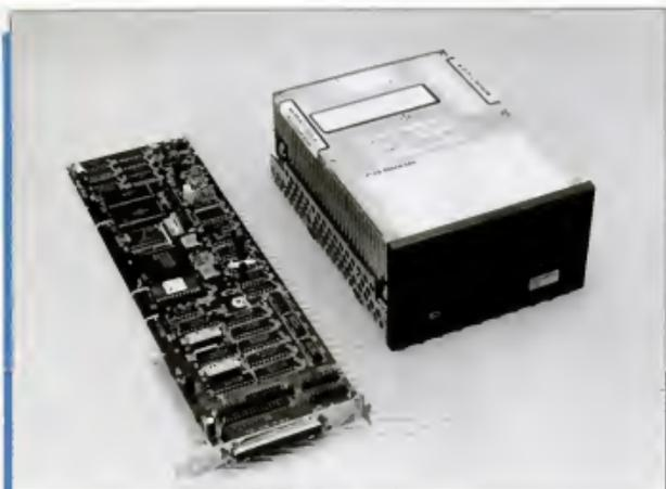
*The Tallgrass TG-5525i is an easily installed internal hard disk that increases capacity by storing a whole track as a single long block of information.*
