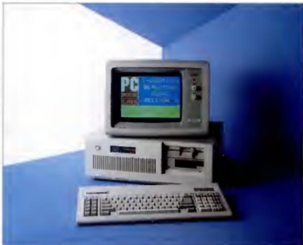
Its 12-MHz processor and 100-nanosecond dynamic RAM chips distinguish the PC's Limited 286 12 from the crowd, as does the SmartVu, a unique front display panel that can help you quickly pinpoint the problem if you have trouble with the machine.
