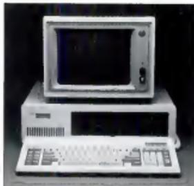
Actually, there's a lot more. Like a built-in clock/calendar with battery back-up, support for an optional 8087 math coprocessor, RAM disk software, a print spooler (along with several useful public domain programs) and a hinged, metal XT-style case with six expansion slots.
