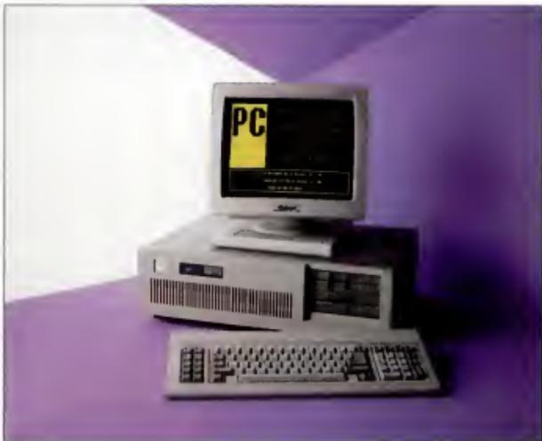
The Tech PC AT Desktop is attractively priced—\$1,399 buys you an 80286-based system unit, a floppy disk drive, a keyboard, and a disk controller card. A toggle switch lets you switch the microprocessor's clock speed between 6 and 8 MHz.
