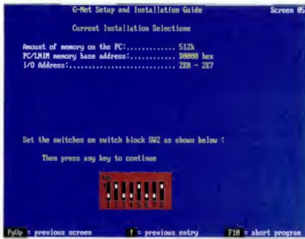
Gateway Communications' installation program simplifies the process of configuring the network interface card by using easy-to-follow diagrams (see screen shot above) to show you how to set the card's switches.
