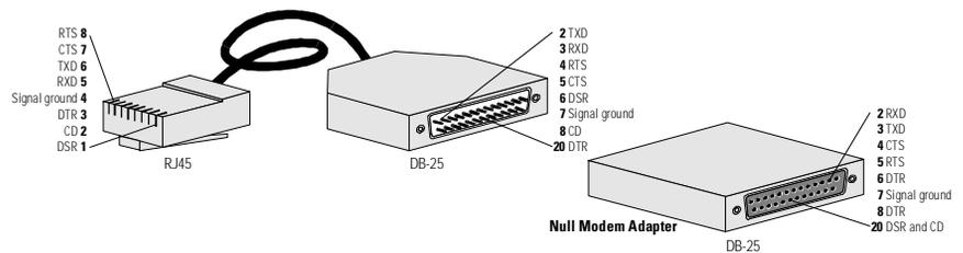
Pinouts for the serial cable [8-pin RJ-45 jack, DB-25 (male), DB-25 (female) with adapter]
