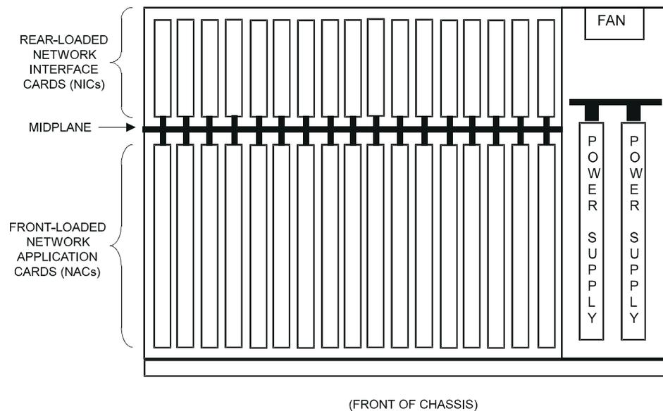
Figure 3. 35 and 45A AC and DC Chassis (Top View)
