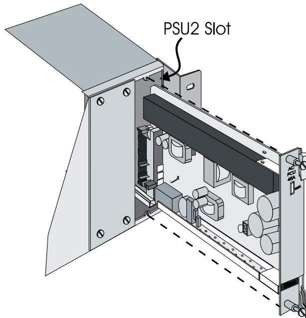
Figure 28. Installation of PSU
