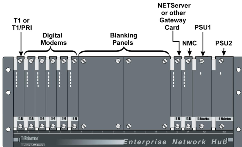
*Figure 5. Typical Digital Configuration
