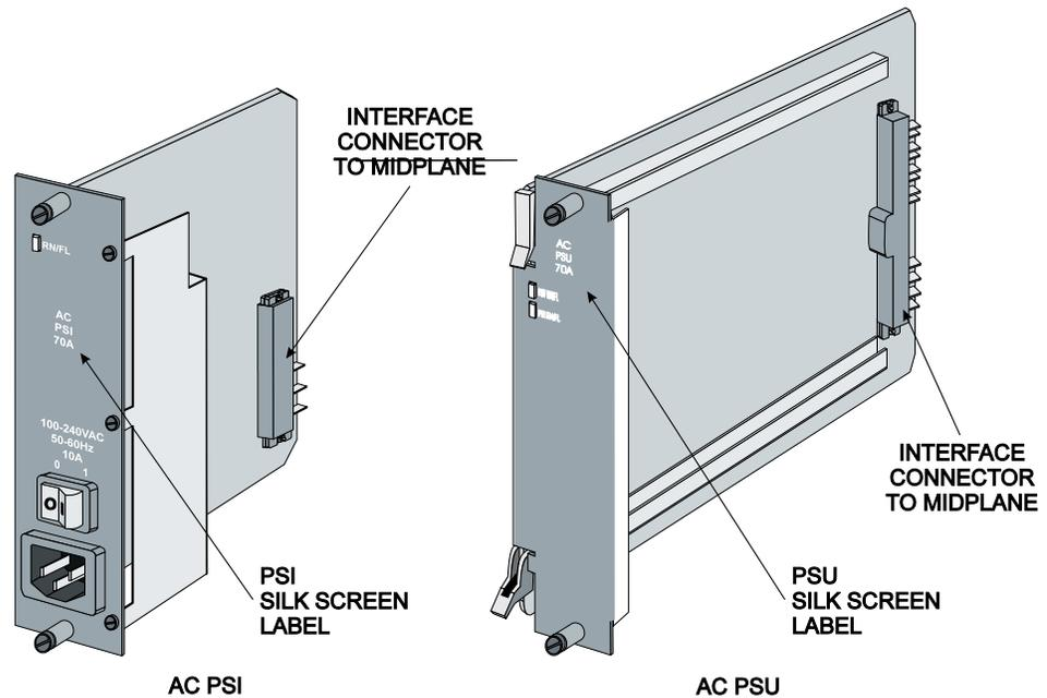
Figure 11. AC PSU and PSI
