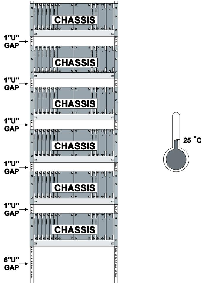
Figure 6. Optimal Rack Installation
