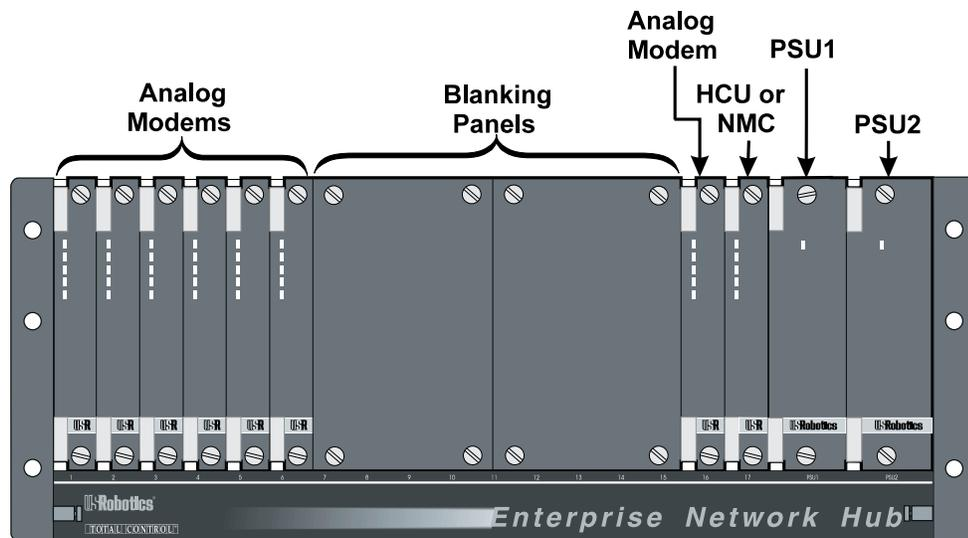
Figure 4. Typical Analog Chassis Configuration
