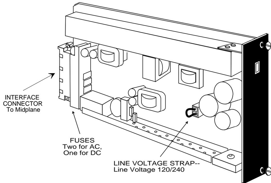
*Figure 26. Line Voltage Strap and Fuse Locations*
