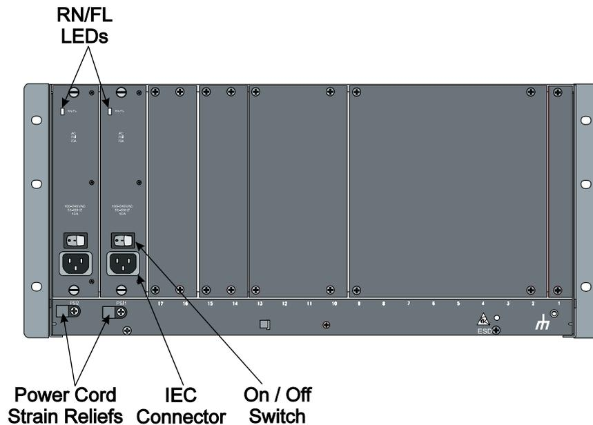
Figure 15. AC Chassis Rear Panel
