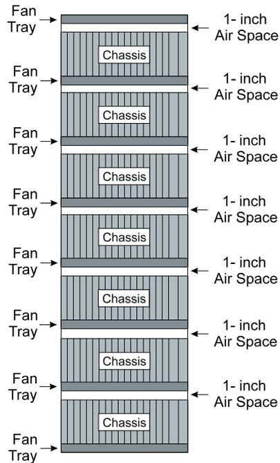
*Figure 24. Equipment Rack with Fan Trays*
