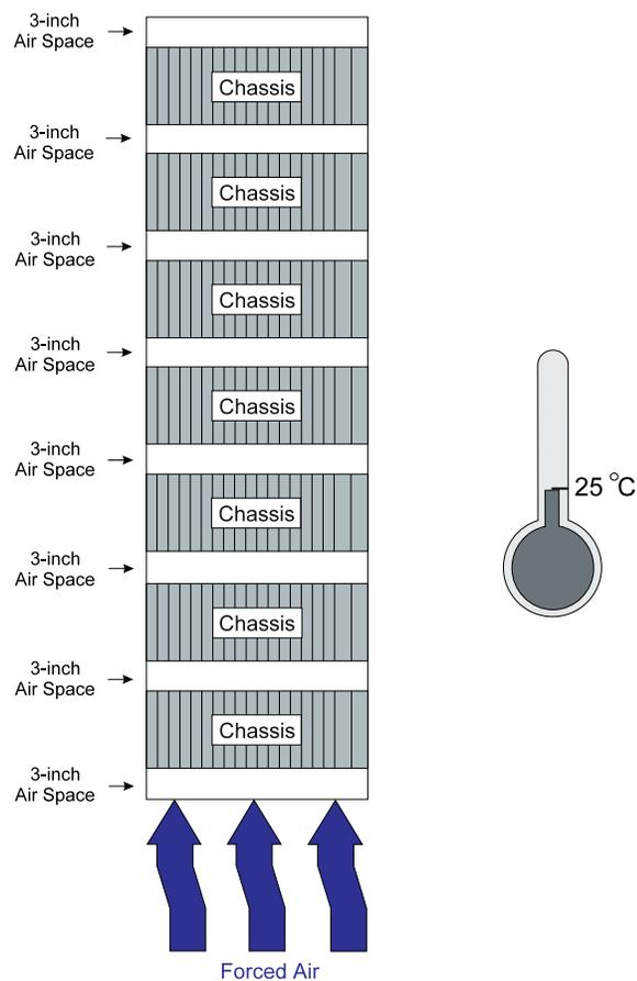
*Figure 19. Optimal Rack Installation Without Fan Trays*
