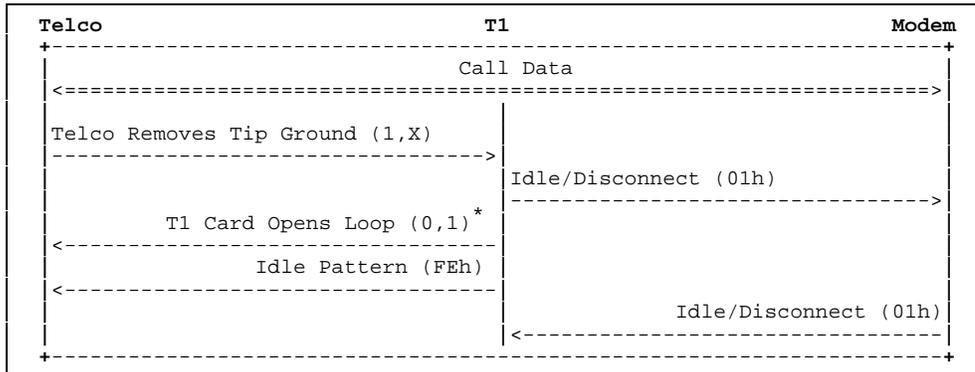
\*The T1 Card must send this (0,1) signal as soon as possible because the TELCO can present a new call as soon as it removes tip ground.
