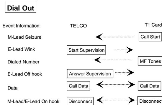
**Figure 3-2. Signaling Between TELCO and T1 Card for a Dial-Out Call**
