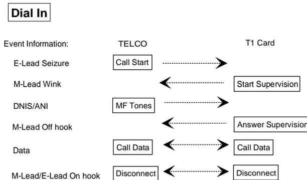
**Figure 3-1. Signaling Between TELCO and T1 Card for a Dial-In Call**
