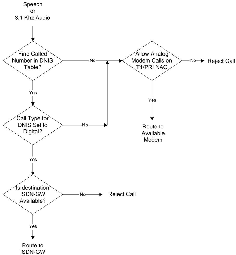
Figure 6-2. Call Routing Through the DNIS Table
