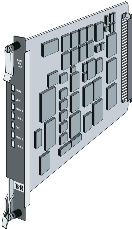
*Figure 3-1. Dual T1/PRI Network Application Card*
