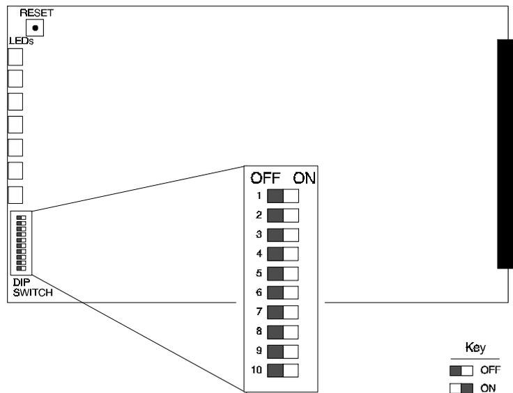
Figure 3-2. Dual T1/PRI NAC DIP Switches
