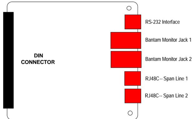
*Figure 2-1. T1 Network Interface Card*
