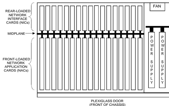
Figure 4-1. Total Control Chassis (Top View)
