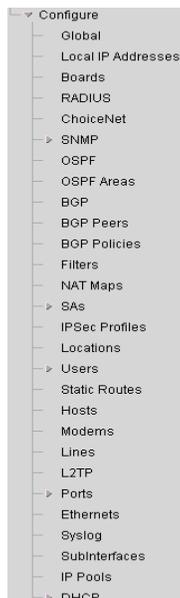
When working with a PortMaster 4 product, you configure functions such as ports and lines by selecting **boards** first. (See “Configuring PortMaster 4 Boards” on page 2-15.)
