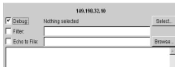
Click the **Select** button on the debug panel to display a new panel allowing selection of debug options (Figure 2-11). Select the category of debug option in the left window. Select one or more specific options in the right window. Click **Set** to enable the chosen options. The selected options appear in the enabled debug window at the top of the panel.
