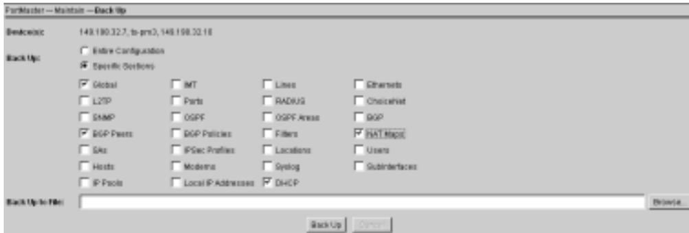
For ComOS 3.8 and earlier releases, restoring from a PMVision backup produces null passwords in the user table. If a user entry has a null password, the PortMaster does not prompt the user for a password at login. As a result, the user might be unable to log in. In addition, an unauthorized user might gain access to the user account because no password is required. Use PMVision or the command line interface to add the user passwords.
