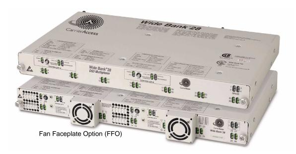
Carrier Access Corporation's Wide Bank 28 DS3 Multiplexer provides a standards-based M13 multiplexing function with TL1 management. This product converts a framed Digital Signal Level 3 (DS3) network connection into 28 Digital Signal Level 1 (DS1) connections to T1 facilities, or into 21 connections to E1 facilities. Each Wide Bank 28 DS3 can be equipped with DS1 cards or E1 cards, but not both.
