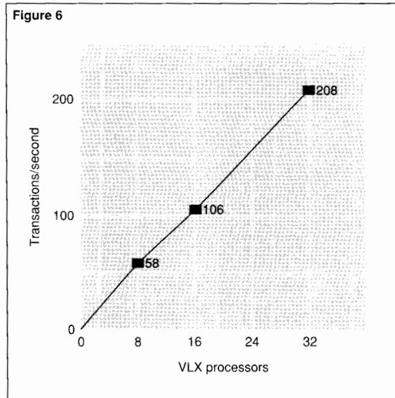
**Figure 6.** OLTP scaleup of NonStop SQL Release 1 on the Debit-Credit OLTP workload. As processors grew from 4 to 32, the database grew from 3.2 million rows to 25.6 million rows, and the terminal network grew from 320 terminals to 2560 terminals. A 26-GB history table was also maintained. The throughput of the system scales almost linearly with the workload.
