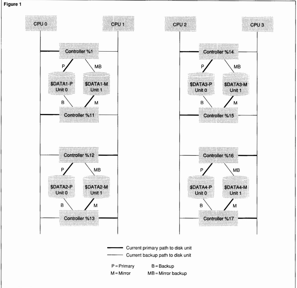
Figure 1 illustrates a configuration consisting of four processors, mirrored disk volumes, and controller pairs. Each disk volume is connected to a separate pair of controllers and controlled by a separate processor. The mirrored volumes are also configured so that the Tandem Disk Process 2 (DP2) can perform parallel reads and writes. The examples in this article use the configuration shown in Figure 1.
