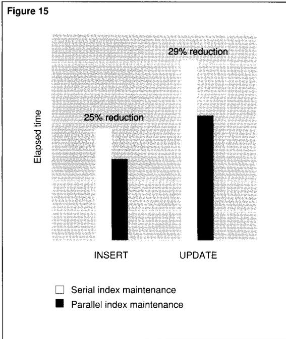
Figure 15 shows the results of an experiment comparing the serial and parallel insertion of 10,000 rows into a table with four indexes. The results demonstrate that NonStop SQL, operating on a disk configuration that promotes parallel index maintenance, significantly reduces the elapsed time of SQL operations in both batch and OLTP applications.
