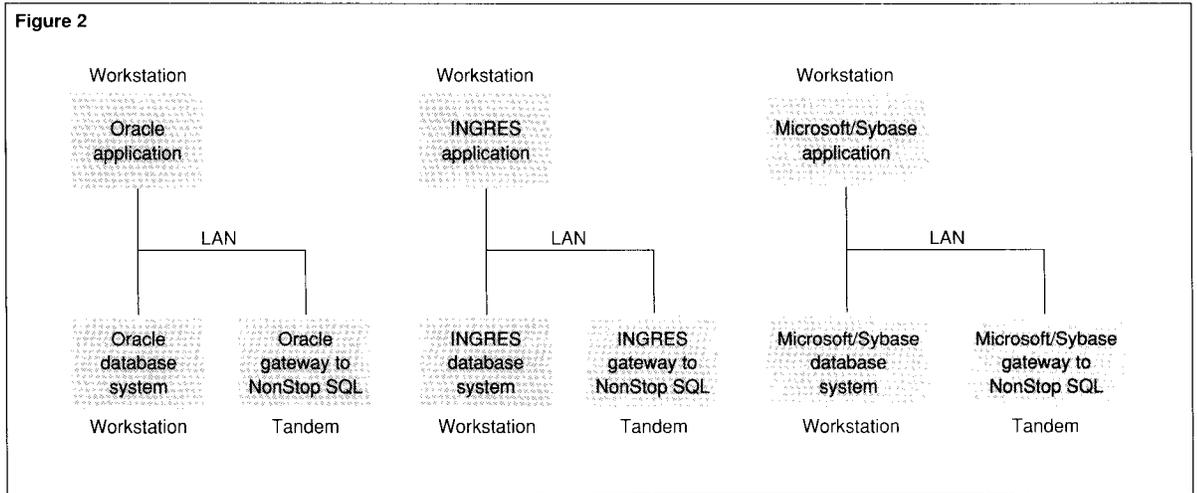
Figure 2 shows examples of gateways to Nonstop SQL. An Oracle application can access an Oracle database directly or a NonStop SQL database through a gateway. In this case, Oracle is the client system and NonStop SQL is the server system. Similarly, an INGRES or Microsoft/Sybase SQL application can make the same calls to its own SQL database or to a NonStop SQL gateway. In this case, INGRES or Microsoft/Sybase is the client system and NonStop SQL is the server system.
