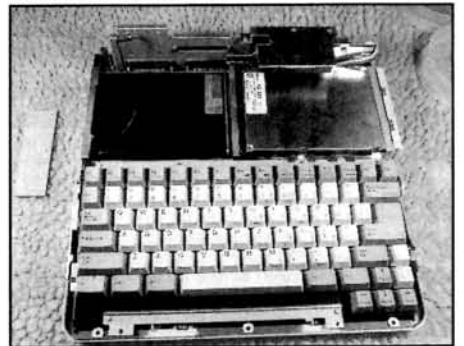
Photo 17 Installing the Keyboard
