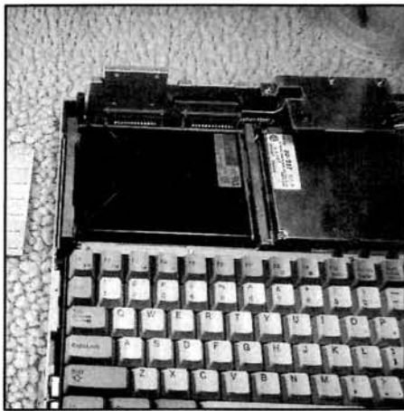
Photo 18 Installing the Cover Plate
