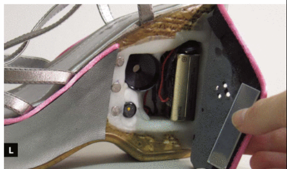
your leather. Fig. K: Mylar pattern for PMP flap includes a cutout for the PMP screen. Fig. L: Completed alarm system with holes punched in leather flap and sheet steel glued to the edge for magnetic closure.
