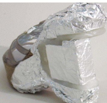
Fig. A: Balsa template for alarm components, wrapped in foil and traced onto heel. Glue this foil so it won't slip. Fig. B: Template and hollowed heel wrapped in foil. Cover exposed parts of the shoe; ShapeLock is tough
