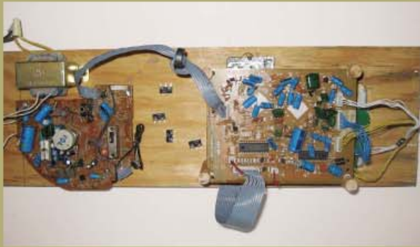
Circuit board and transformer from donor boombox attached to mounting board with standoffs and heat-shrink tubing to prevent shorts.
