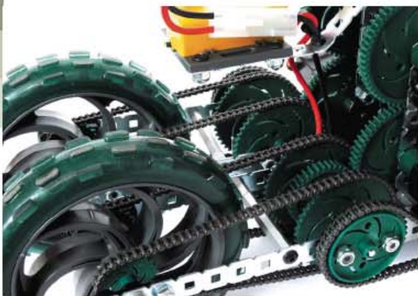
Here's one sophisticated design, the Vex Tomahawk from VexLabs, which originally designed the Vex system. It's a four-wheeled vehicle that uses two servos and differential power to lean into turns, up to 30 degrees, with Segway-like ease.
