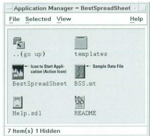
Fig. 2. Contents of an application group for a single application.
