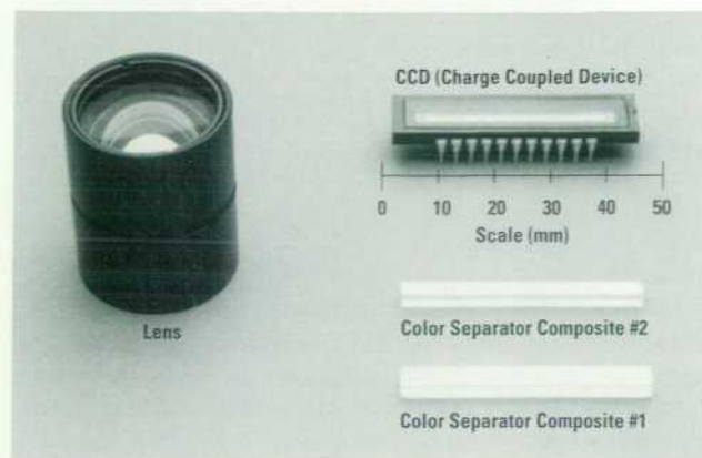
Fig. 4. Lens, CCD detector, and color separator composites.
