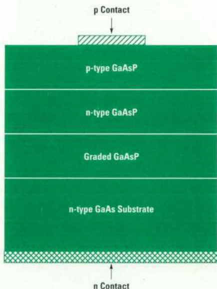
Fig. 1. GaAsP standard red homojunction LED.
