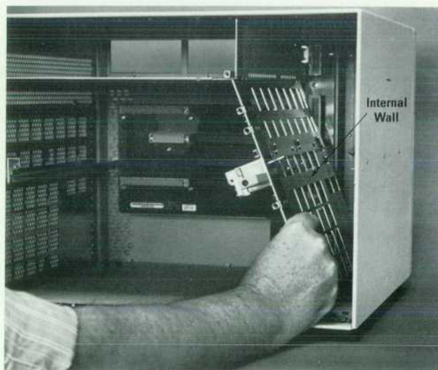
Fig. 3. Gaining access to the Model 747i backplane by removing the internal wall.
