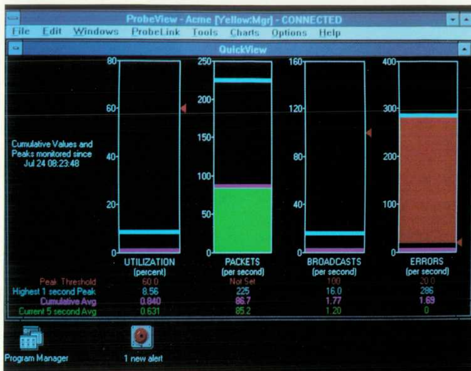
Fig. 2. QuickView shows the current, average, and peak values for packets on the network, bytes on the network, broadcasts, errors, and so on. The network manager can set alarm thresholds for each category.
