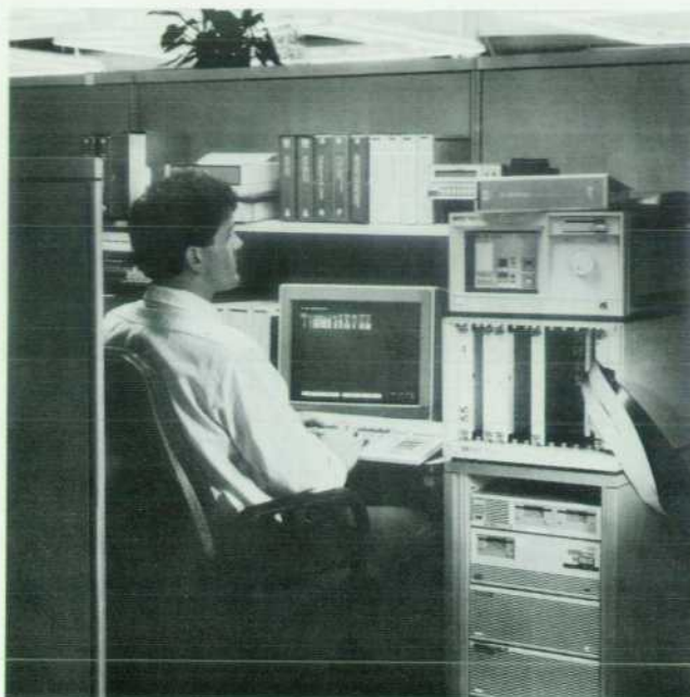
Fig. 2. HP VXIbus development software runs on HP 9000 Series 200 and 300 Computers. It is designed to verify the operation of VXIbus modules and to serve as a learning tool for the VXIbus standard.
