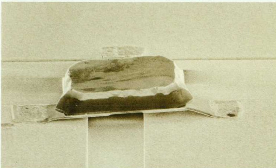
Fig. 12. Photomicrograph of single beam-lead diode mounted on a coplanar waveguide structure for nonlinear and linear testing at microwave frequencies.
