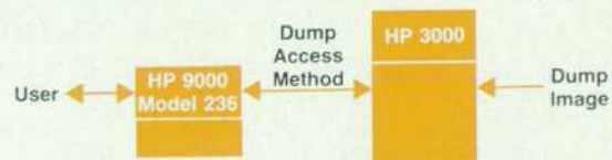
Fig. 2. AIDA runs on an HP 9000 Series 200 Workstation. A process on the HP 3000 called the dump access method sees the workstation as a terminal.
