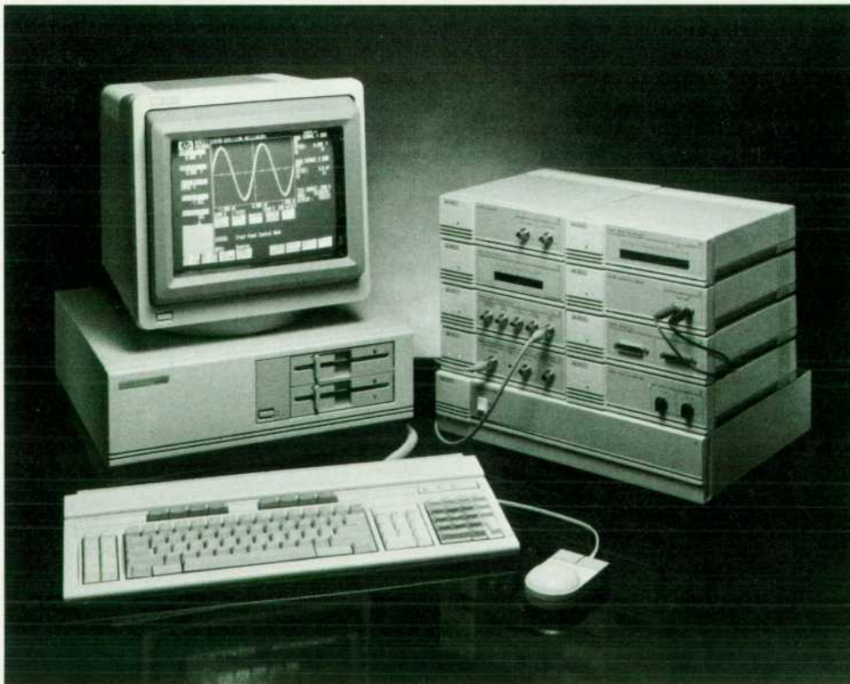
Fig. 1. The HP PC Instruments system is designed to work in concert with the HP Vectra and HP 150 Computers and the IBM PC/XT/AT computers. Eight different instruments, offered in modular, stackable cases, and several software packages and accessories are available. A single interface card will support any combination of up to eight modules. More instruments can be added by using additional interface cards.
