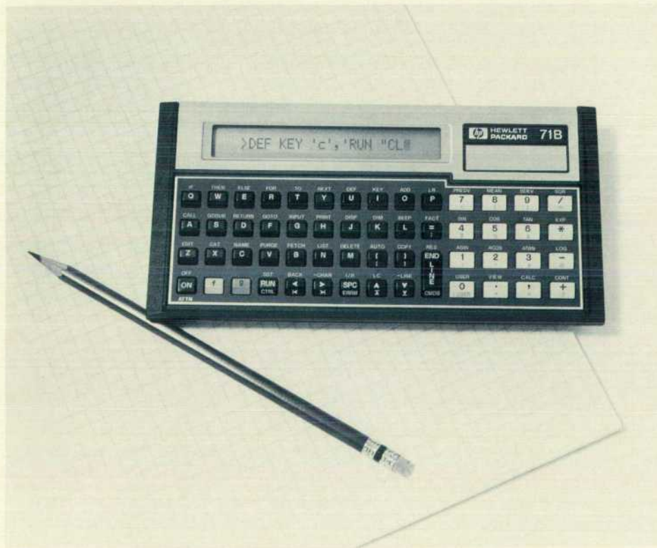
Fig. 1. The HP-71B Computer is HP's latest and most powerful handheld computer. Intended for use by the technical professional, it can be used as a highly advanced algebraic calculator and/or as a computer using a built-in 240-keyword BASIC programming language. Four ports allow addition of more RAM and/or ROM to expand system memory and to enhance the HP-71B's computational power. An optional hand-pulled card reader module can be added for local portable mass storage and an HP-IL module can be added for communication with peripherals and instruments.
