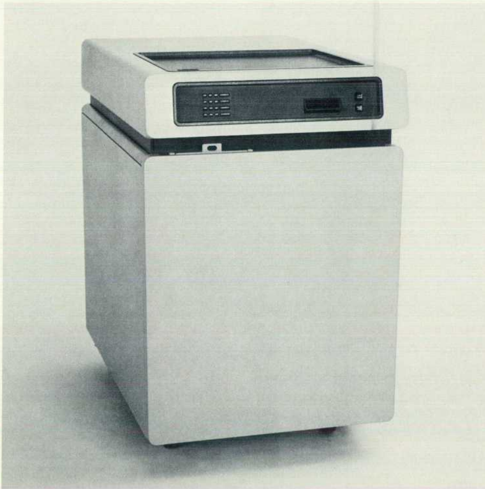
Fig. 1. The HP 7933 and 7935 Disc Drives are 404-megabyte drives that feature data error correction and extensive diagnostics. Externally, the drives are identical. The difference is that the 7935's disc pack can be removed and replaced by the user.
