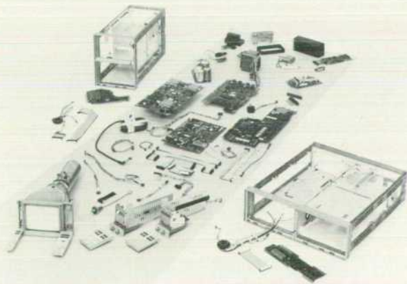
Fig. 2. Modular design approach results in modules small enough to have the same interface and coupling relationships in both configurations. Only one circuit board, the interface board, differs between the two 1980A/B models.
