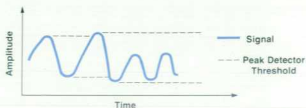
Fig. 5. When the signal maxima and/or minima change as shown, the peak detectors must be reset frequently to correctly detect signal peaks.
