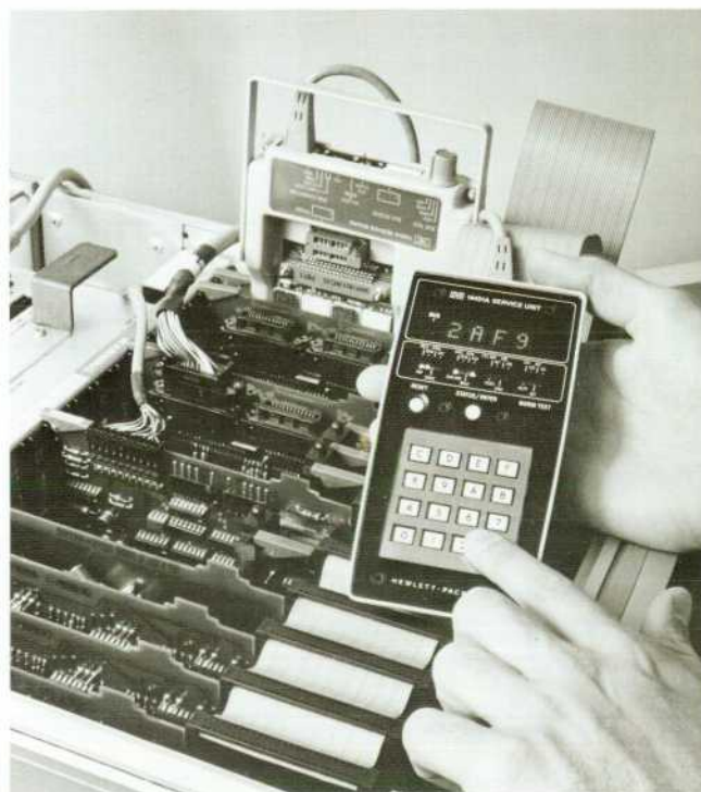
Fig. 4. The 14451A Service Circuit-Analyzer-Board allows service personnel to exercise additional facilities in the system to aid in identifying a failure.
