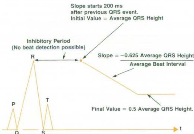
Fig. 3. Graph of the cardiometer threshold for detecting heart beats. The inhibitory period imposed after a beat is detected reduces the possibility of counting the T portion of the waveform as a separate beat.
