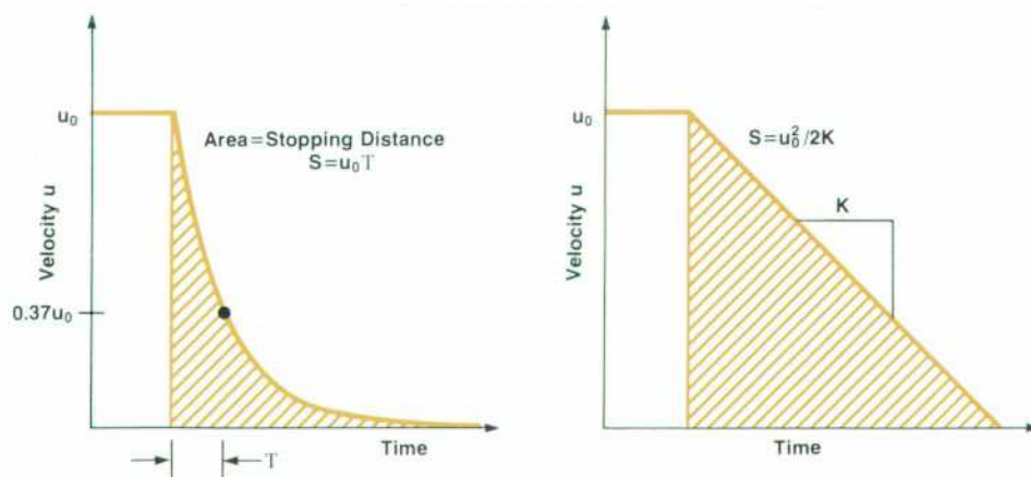
Fig. 9. Two types of braking phenomena are present in non-linear systems. Total stopping distance S is a superposition of the two mechanisms: S_T = Gu_0 + Hu_0^2 , where G and H are constants.
