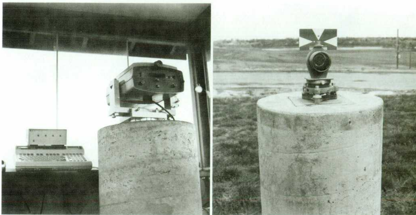
Fig. 16. Equipment used to monitor earth movement includes stable mountings for both the 3850A and the retroreflector.
