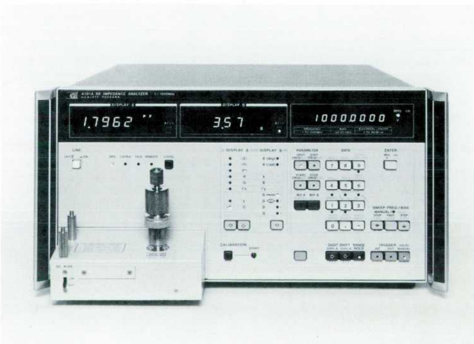
Fig. 1. Model 4191 RF Impedance Analyzer measures impedances from 1 m \Omega to 100 k \Omega at frequencies from 1 to 1000 MHz. Measurements are accurate within 0.5% to 2% of reading. The analyzer has frequency sweep capability, 4½-digit resolution, built-in dc bias with sweep capability, high stability, and a selection of versatile test fixtures.
