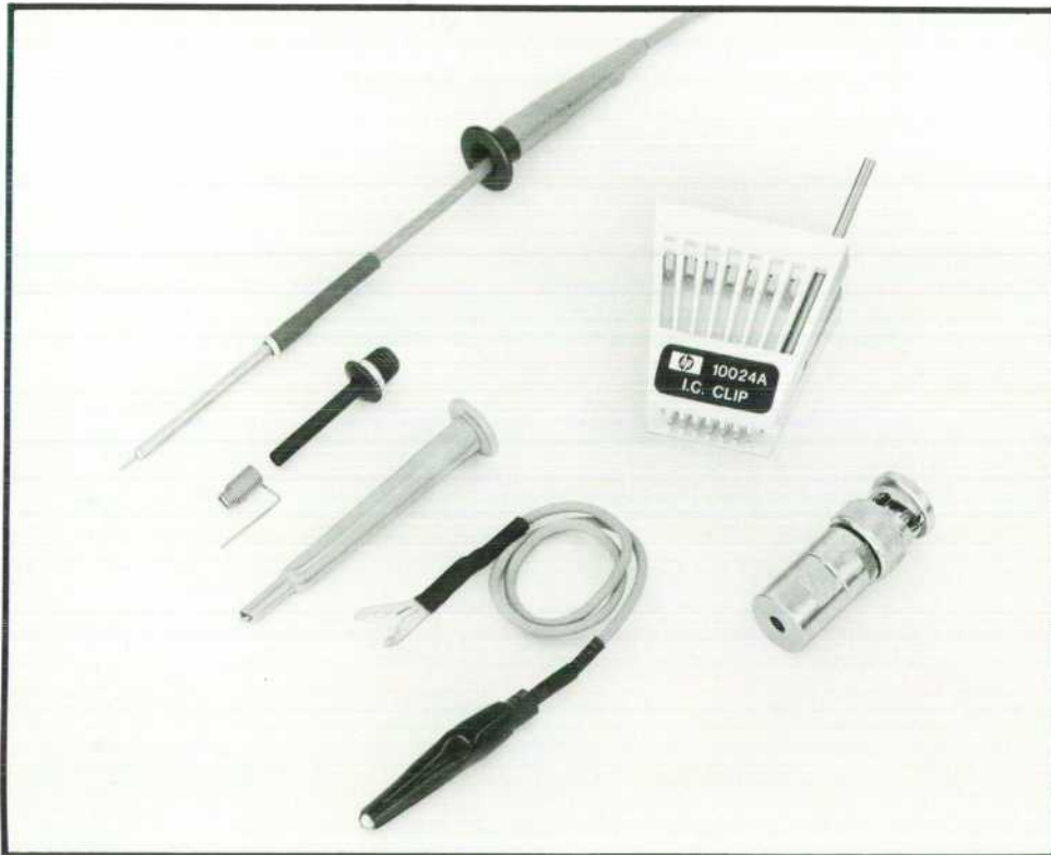
Fig. 1. New miniature oscilloscope probe (right) is shown here alongside a conventional probe (left) of recent design. The 2.4-mm (0.1-inch) diameter of the new probe permits probing where device leads are on 0.1-inch centers.
