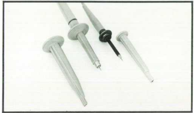
Fig. 1. New miniature oscilloscope probe (right) is shown here alongside a conventional probe (left) of recent design. The 2.4-mm (0.1-inch) diameter of the new probe permits probing where device leads are on 0.1-inch centers.
