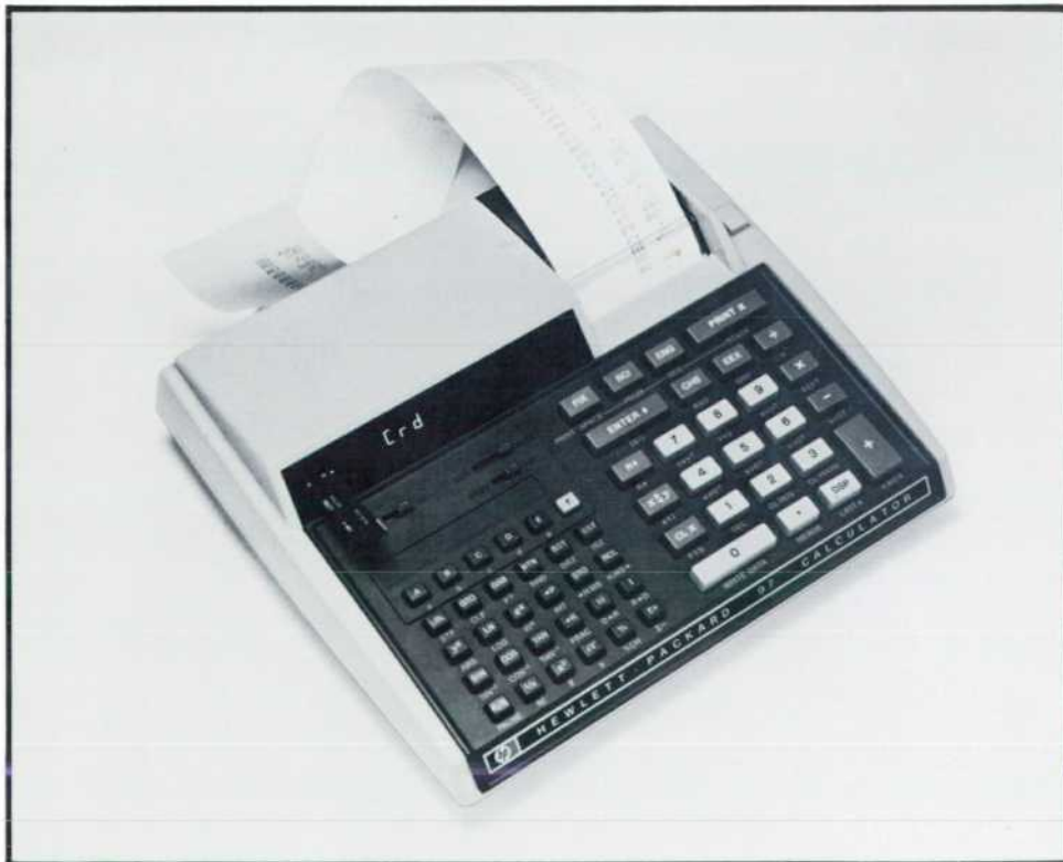
Fig. 2. HP-97 is a fully-programmable printing calculator that fits in a standard attache case. It weighs only 1.13 kg including battery pack.
