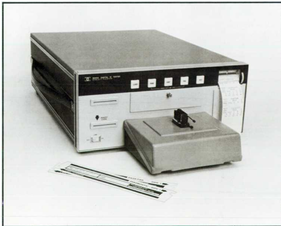
Fig. 1. Model 5045A Digital IC Tester is programmed by means of factory-prepared prerecorded magnetic cards to test a wide variety of commercially available digital integrated circuits. A built-in printer provides a record of test results and failure analyses.
