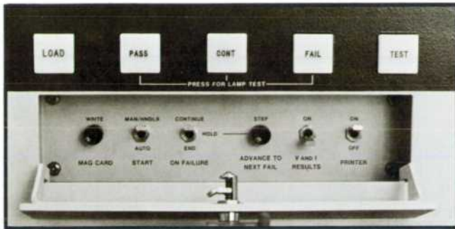
Fig. 5. The V AND I RESULTS switch causes the tester to vary the voltage and current on failed pins until the device passes and then print those voltage and current readings. See Fig. 6.
