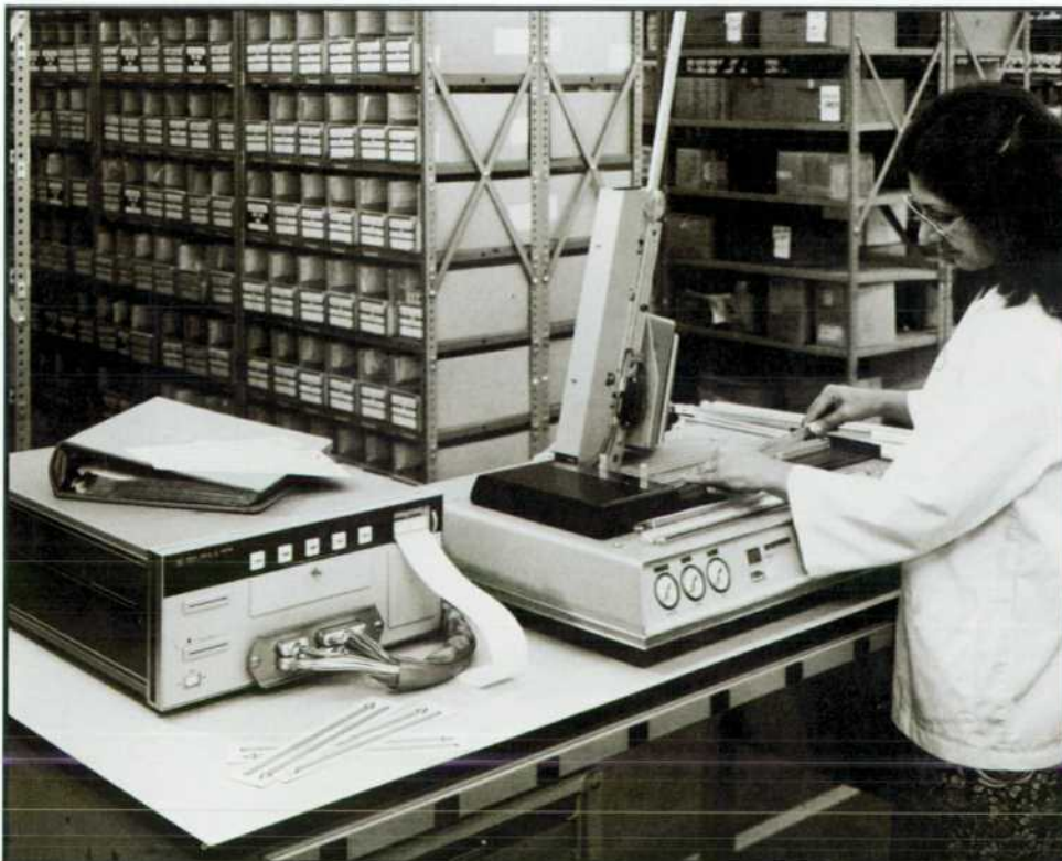
Fig. 7. The test deck of the 5045 IC Tester can be removed and mounted on an automatic handler. Interface electronics are available for many commercially available handlers.
