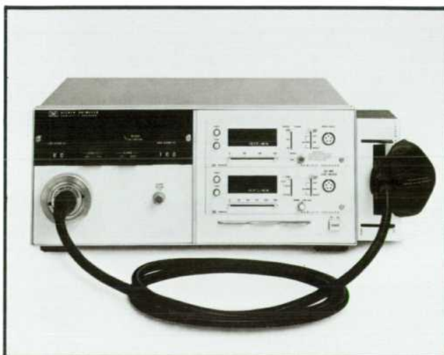
Fig. 7. Oximeter has space for optional patient-monitoring modules to give simultaneous measurements of heart rate, pressure, temperature, or respiration. Standardization cavity then mounts on the side of the instrument.
