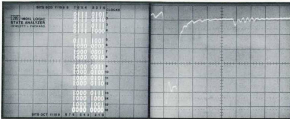
Fig. 5. Trigger word here is set to end the display, showing that the two-decade BCD counter resets on 89 rather than 99. Resetting the Logic State Analyzer to trigger on 88, and using the trigger output to start an oscilloscope (right), discloses a "glitch" on the reset bus on state 90.
