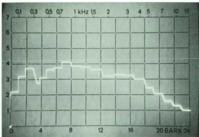
Fig. 5. Typical loudness analyzer display in CHECK mode. In this mode, analyzer input comes from built-in wideband noise generator.
