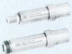
Fig. 1. New -hp- Models 10457A-8A 50-to-75-ohm adapters simplify testing of 75-ohm systems with -hp- Model 1415A Time Domain Reflectometer. Adapters are 25-ohm resistors with one GR874 connector and one type 'N' or 'F' connector.
