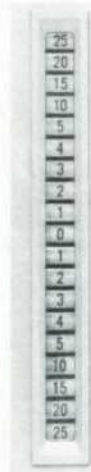
Fig. 9. Position of zero level baseline selected by Positioning control is indicated by illuminated numerals, enabling measurement of dc levels with analog voltmeter accuracy even with zero level displaced up to \pm 25 cm from center screen.
