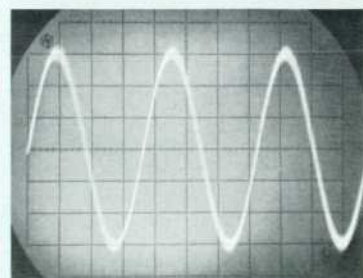
Fig. 2. Oscillograms, made with Differential Amplifier plug-in operating while dc-coupled on most sensitive range (50 \mu V/cm), demonstrate absence of drift over extended periods. Time elapsed between first and second oscillograms was 65 hours but there is no discernible drift in dc level of CRT trace.
