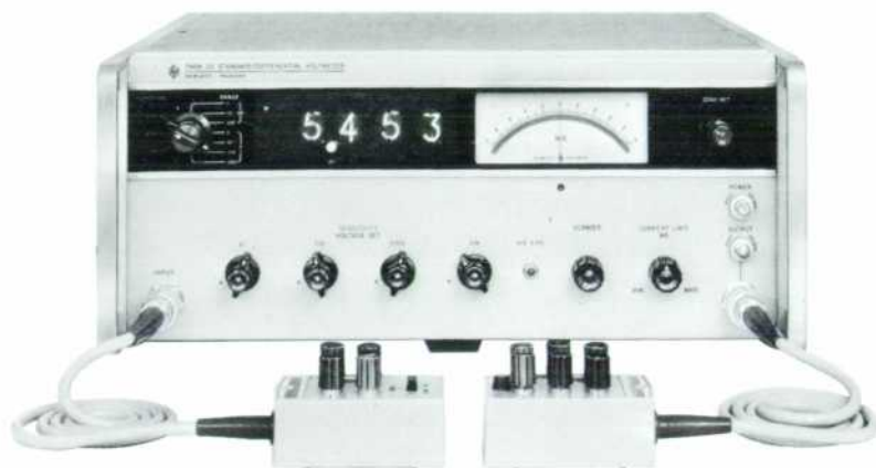
Fig. 2. DC Standard/Differential Voltmeter has illuminated numerals to show settings of corresponding decade divider Voltage Set controls. Range switch sets decimal point in display and illuminates corresponding units of measurement (volts or millivolts). Push-button Sensitivity knobs concentric with Voltage Set controls connect meter to corresponding decade of resistive divider and adjust sensitivity of meter accordingly. Operator is able to make differential voltage measurement quickly by depressing Sensitivity push-button for most significant digit first, bringing meter near null with that Voltage Set control, then proceeding with other digits in turn.
