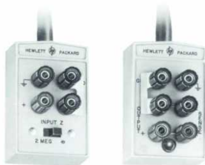
Fig. 9. Connections to and from new instrument are made through connector boxes on detachable cables. Input connector box has two guarded and floating input connectors and connections to guard shield and circuit ground. Switched 2-megohm resistor provides discharge path for input capacitance (low leakage of high-impedance input retains charge for some time after removal of source).
