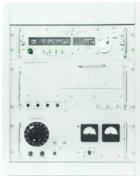
Fig. 4. Panel view of one of "atomic" clocks used in experiment. Cesium standard in middle drives electronic clock (top) which integrates standard frequency and also produces very accurate electrical "ticks" based on driving frequency. Power supply unit at bottom provides for operation from a range of ac and dc voltages.
