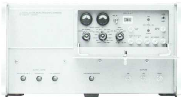
Fig. 7. Front view of Cesium Beam Frequency Standard. Cesium beam standards utilize a quantum-mechanical effect to produce ultra-stable frequencies. Two standards were combined with electronic clocks and power supplies to form an "atomic" clock with stabilities of a few parts in 10^{12} .
