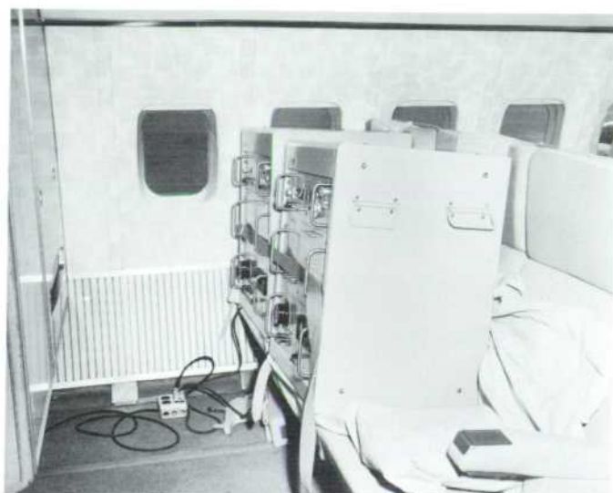
Fig. 2. The two atomic clocks being fastened in passenger seats aboard airliner. Operating power in flight was supplied by plane.
