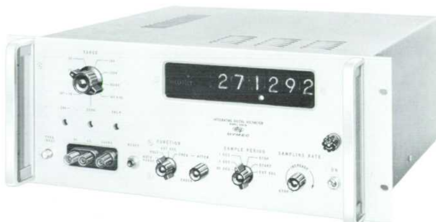
Fig. 3. Dymec Model 2401B Integrating Digital Voltmeter has internal calibration source with stability of \pm 0.01\% per six month period to match voltmeter's high accuracy. Programmable voltmeter has five ranges, from \pm 0.1 to \pm 10000 v full scale, with 300% overranging on four most sensitive ranges for increased resolution and sensitivity on 1-to-3 readings. Guarded, floating input provides high common mode noise rejection; integrating operation averages out superimposed noise and completely eliminates effect of power line hum to retain high accuracy in presence of noise. Overall instrument common-mode rejection is 140 db (10 million to 1) at all frequencies, including dc.
