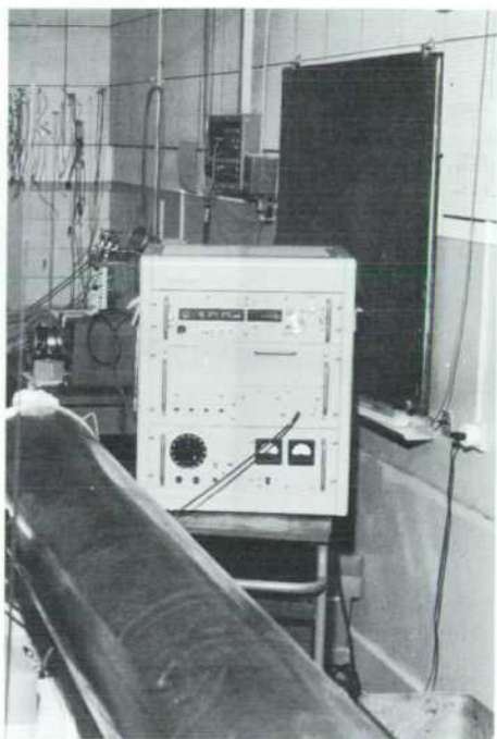
Fig. 5. Frequency comparison being made between one standard and the "long" cesium beam standard (foreground) at the Laboratoire Suisse de Recherches Horlogeres, Neuchatel, Switzerland. This long standard is considered one of the world's best cesium standards.
