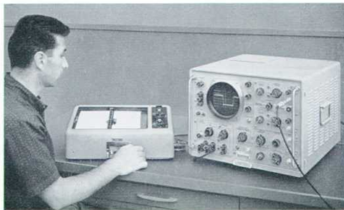
Fig. 1. New -hp- militarized oscilloscopes are designed with plug-in units for horizontal as well as vertical system, thus achieving increased flexibility. Illustration shows oscilloscope being used with one type of horizontal plug-in that enables oscilloscope display to be recorded on external X-Y recorder.
