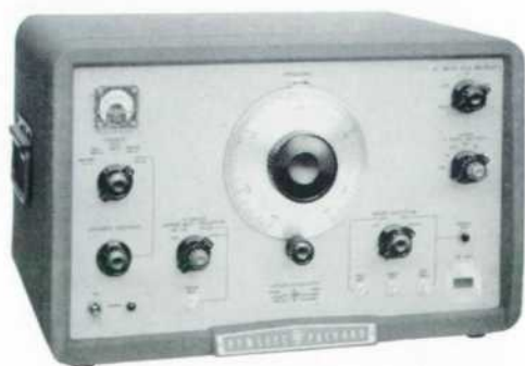
Fig. 1. New -hp- Model 686A voltage-tuned sweep oscillator provides c-w, f-m, a-m and swept outputs over 8.2 - 12.4 kmc range. Sweep widths as wide as full band can be selected at a wide range of rates to suit measurement conditions.
