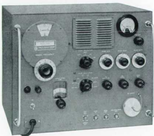
Fig. 1. New -hp- Model 626A SHF Signal Generator has high power output over 10 to 15.5 kmc range, is provided with direct-reading frequency dial and output attenuator, has flexible modulator.
