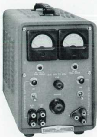
Fig. 1. hp Model 711A Regulated Power Supply has many operating features such as overload relay, voltage vernier that suit it to everyday use.
