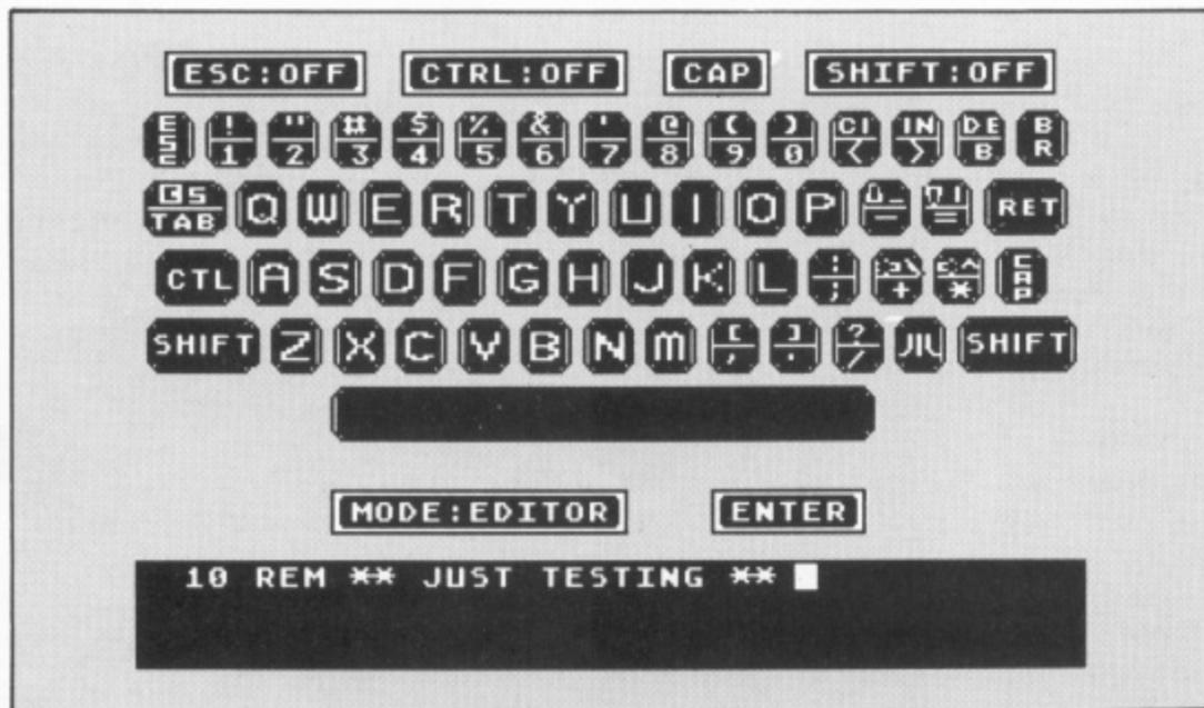
Figure 1: Using the touch tablet as a keyboard
